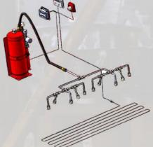
Fully **Automated** Customized Fire **Extinguishing Systems**
